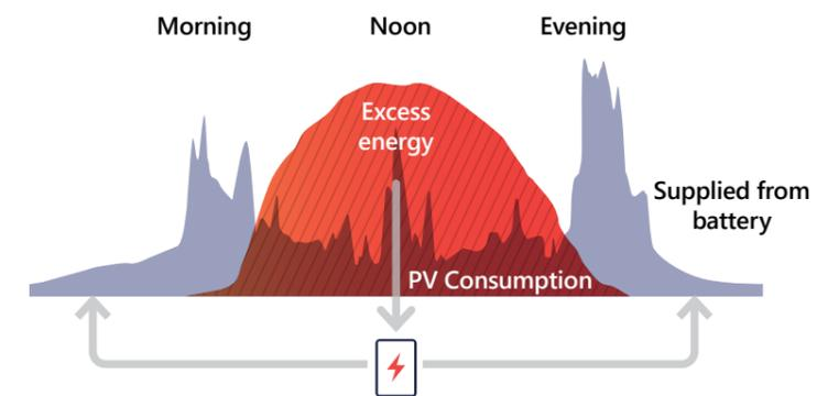
With StorEdge, the excess energy produced during peak sunlight hours is stored to the battery and used later so no energy is ever wasted.
